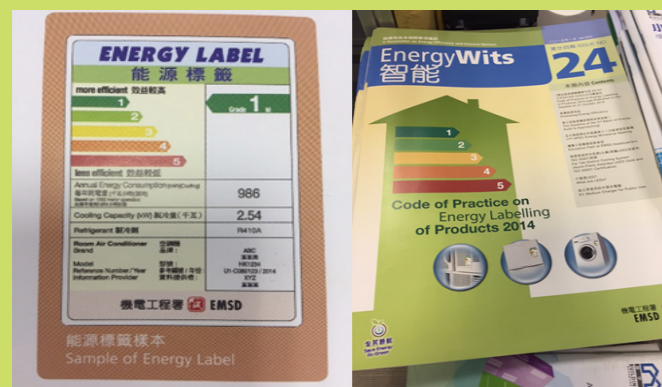
Figure 4.2.14 Sample of an energy label and the newsletter "Energy Wits" on energy efficiency and related matters from the Electrical and Mechanical Services Department (EMSD) available at EMSD: http://www.energylabel.emsd.gov.hk/en/mainpage.html
