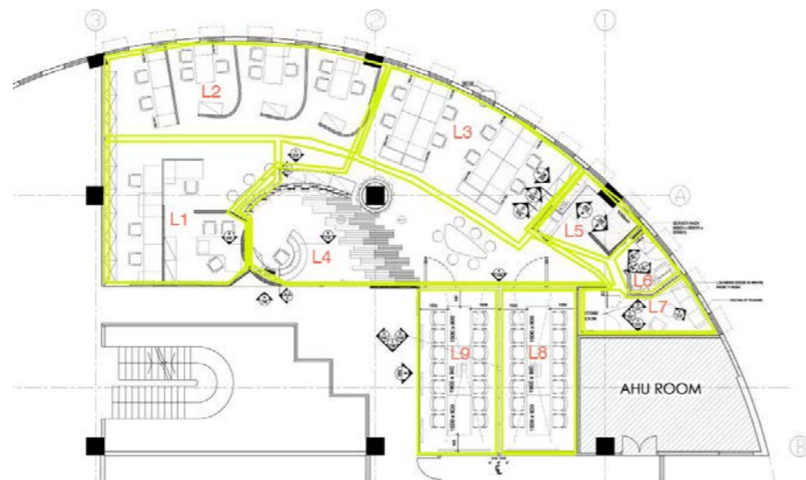
Figure 3.2.5 Lighting zone of the Hong Kong Green Building Council office (Source: Hong Kong Green Building Council)
