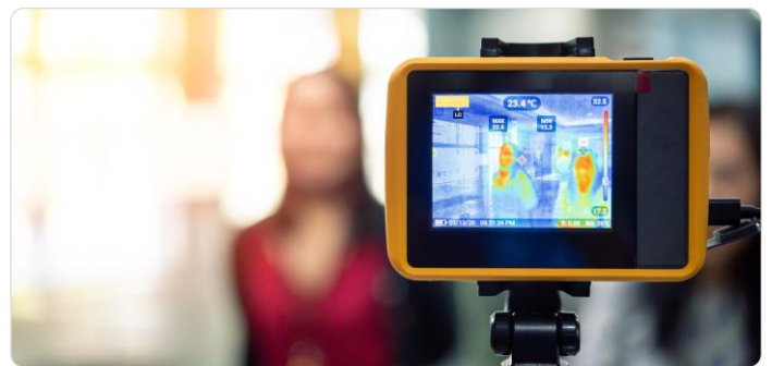
Figure 109: Smart Temperature Sensors and Thermostats Thermal imaging system to measure surface skin temperature.
