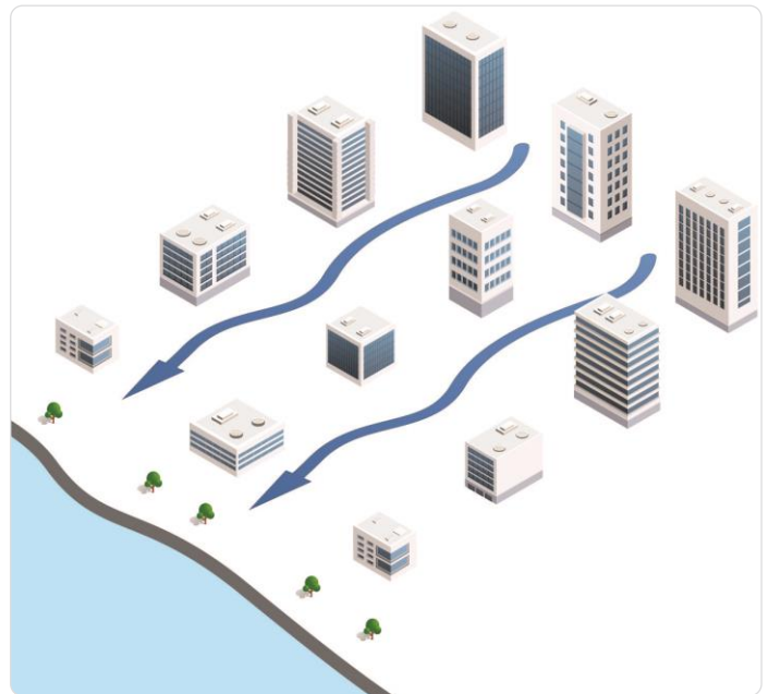
Figure 105: Gradation of Height Profile Consideration of height profile and breezeways in an area.
