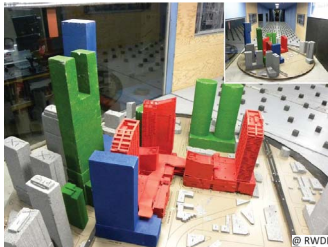
Figure 8: Wind tunnel test to measure building performance under various dynamic buffeting conditions
