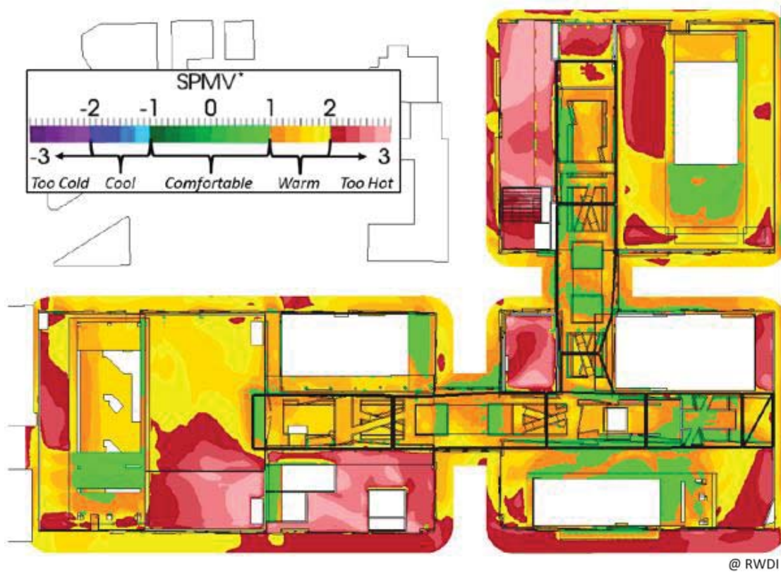
Figure 6: Thermal dynamic simulation results showing the thermally comfortable zone created underneath Climate Ribbon™ [At mid-day in summer period]
