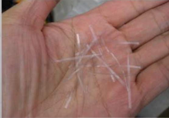
Close up of synthetic macro-fiber
