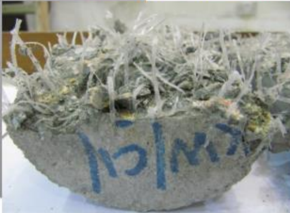
Close up of fibers at fracture surface
